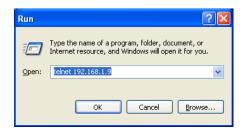
The **Telnet** window will open and the **Server** screen will appear. See chapter 9 for configuration screens and navigation.
